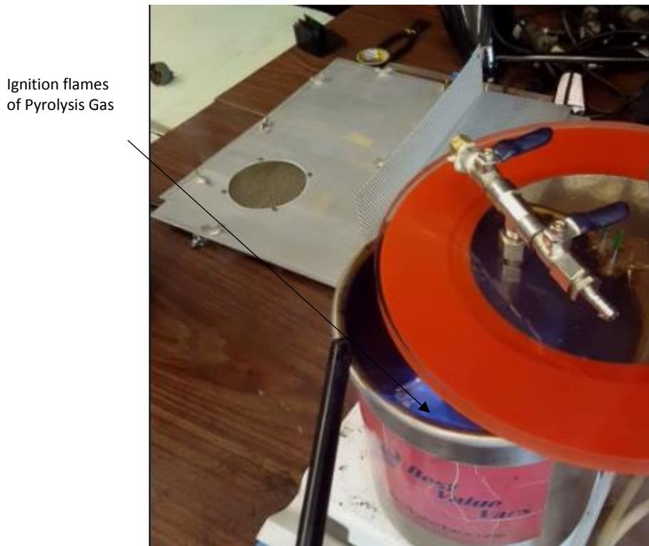
Figure 7- 6. Ignition test of hydrocarbon gases from pyrolysis reaction
