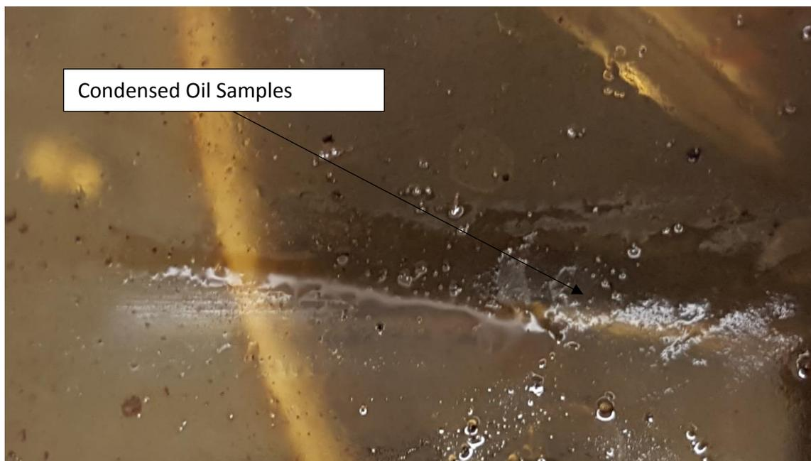
Figure 7- 2. Condensed oil sample on the reactor lid from a 15 g LDPE thermoplastic
